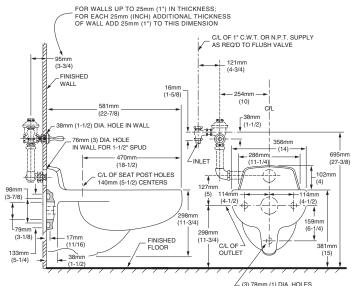
(3) 78mm (1) DIA. HOLES FOR CARRIER STUDS
